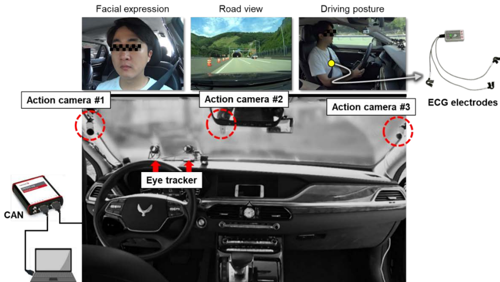
Figure 6.1. Driver cockpit for the on-road evaluation of passive task-related fatigue of the driver
